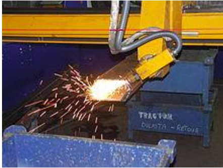
Plasma cutting with a tilting head
