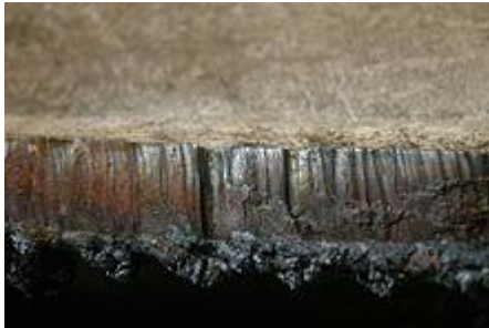
Freehand cut of a thick steel plate
