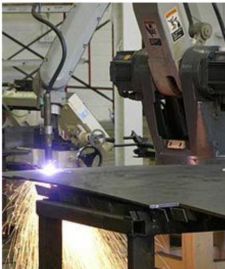
Plasma cutting performed by an industrial robot
